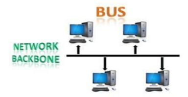
The bus topology is designed in such a way that all the stations are connected through a single cable known as a backbone cable.  $\circ$  Each node is either connected to the backbone cable by drop cable or directly connected to the backbone cable.  $\circ$  When a node wants to send a message over the network, it puts a message over the network. All the stations available in the network will receive the message whether it has been addressed or not.
