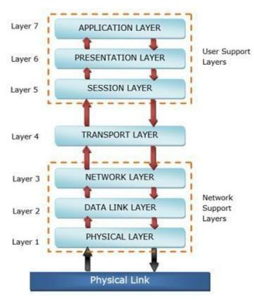
The physical layer, data link layer and the network layer are the network support layers. The layers manage a physical transfer of data from one device to another. Session layer, presentation layer, and application layer are the user support layers. These layers allow communication among unrelated software in dissimilar environments. Transport layer links the two groups.
