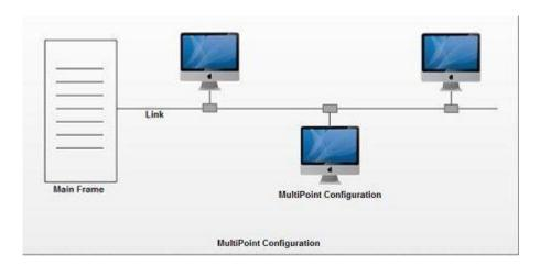
Broadcast network provides the provision for broadcasting & multicasting. Broadcasting is the process in which a single packet is received and processed by all the machines in the network. It is made possible by using a special code in the address field of the packet. When a packet is sent to a subset of the machines i.e. only to few machines in the network it is known as multicasting.
